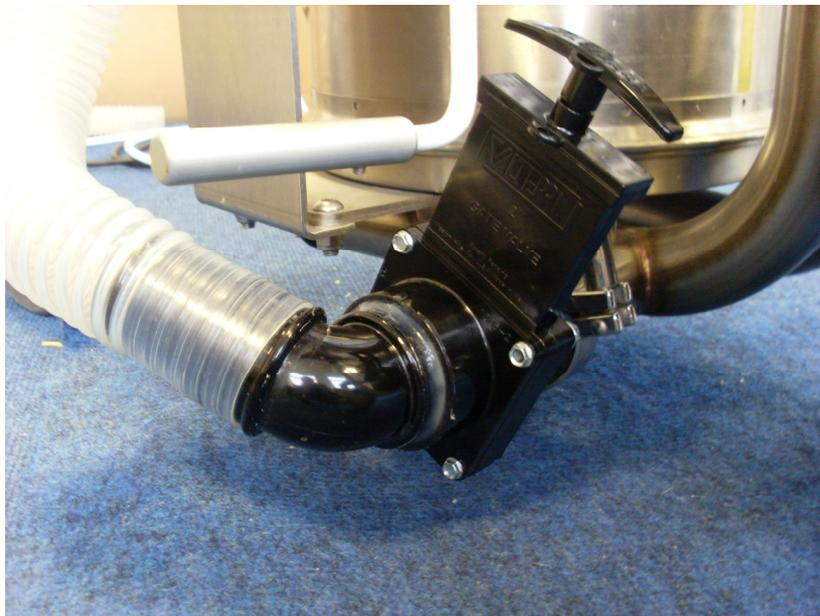
Pulling the lever upwards immediately connects the manual breathing circuit to the main patient circuit.
