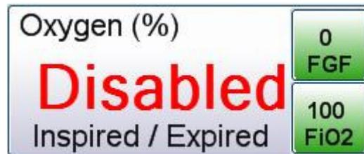
Note that the Oxygen value is shown as Disabled at start-up until the unit has initialised. The feature will not work unless the oxygen sensor has self-calibrated and the Oxygen levels are being measured.
